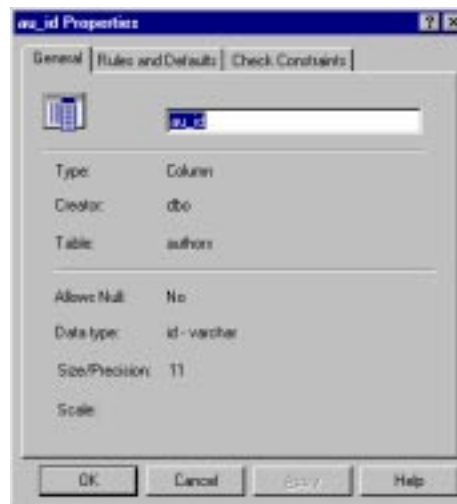
Figure 22-16: Column Properties: General tab
